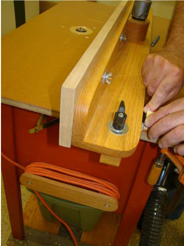
Decent shot of Bill's fence. Oak butt joint frame with MDF split fence face. Common hardware. Here, ill is clamping on a micro adjust.
