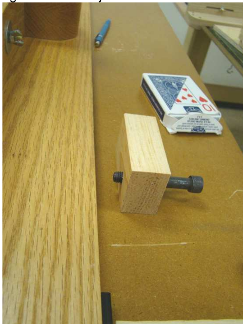
Home made micro adjust. An allen head bolt screwed into a drilled out hardwood block.
