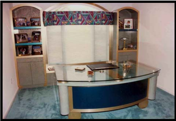
This desk was designed for a client who had deep pockets. There are 5 different types of materials used on this desk. The top is 1/2" thick glass with polished edges.
