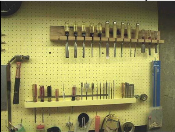
Wooden tool holding racks held to pegboard with toggle bolts.
