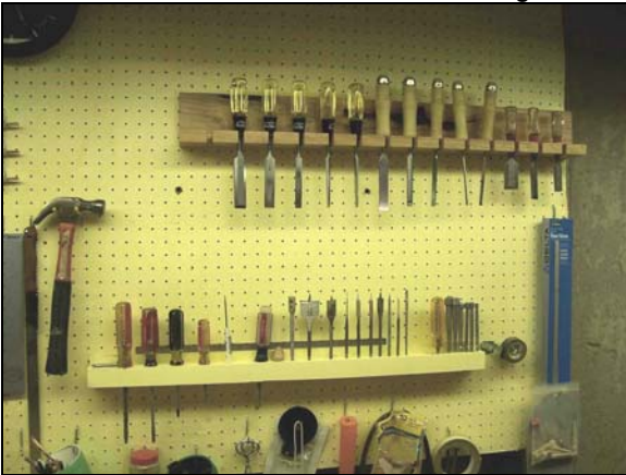
Wooden tool holding racks held to pegboard with toggle bolts.
