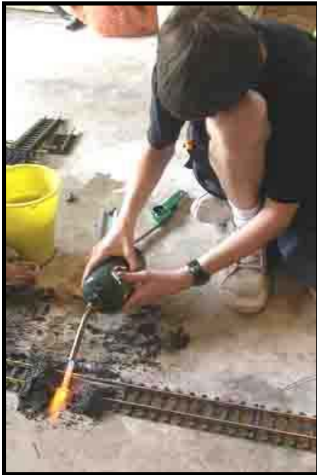
Paul at work soldering sections of track. Note us is using what looks like wet screenings to keep plastic railroad ties from melting.
