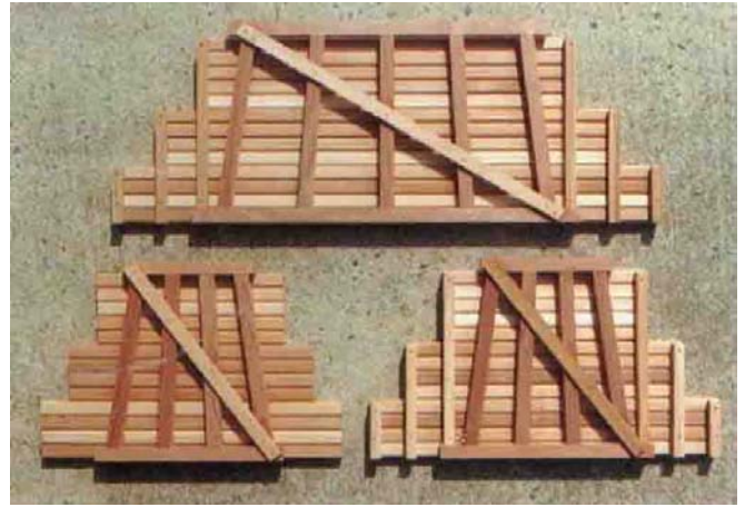
Bridge abutments are built similarly to trestles with solid lumber filling in the space.
