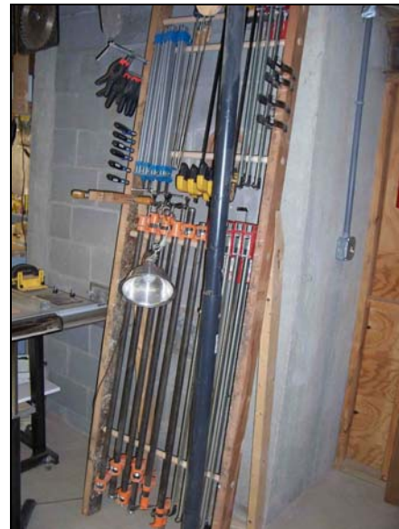
Clamp rack solution in Ron's shop
