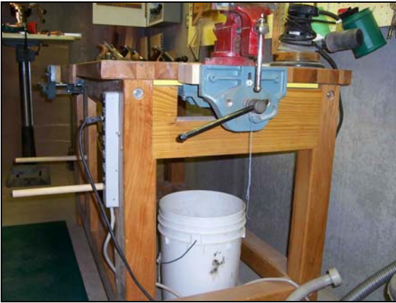
Tail vise pictured here holding a machinist vise for metal work.
