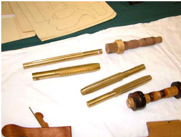
Tap tap tap. Brass taps that Jim made for his work. He makes his own tools in many cases. These are as nice as his planes. Attention to detail....
