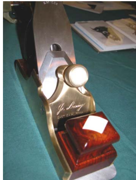
As stated, Jim says there are a lot of other people who make this style plane (called an Infill plane) and some do it better. OK, Jim, I agree. I'd love to take this horrible looking tool off your hands... Just a beautiful tool, an I would bet it works as well as it looks.
