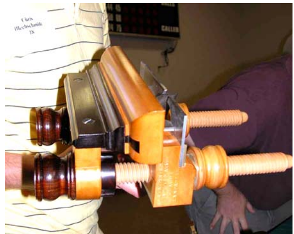
The work on the bottom of the planes is like fine woodworking. This one was originally made by E.W. Carpenter of Lancaster Co., Pennsylvania. Carpenter is noted for his exaggerated nuts and wedge
