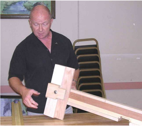
Eoin O'Neill explains the details of the combination jig – table saw fence and router fence.
