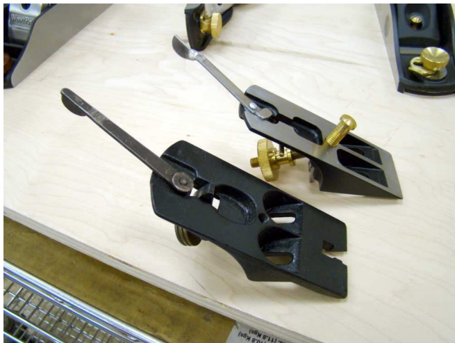
Frogs. They hold the blade and chip breaker, allow adjustments, determine initial angle.
