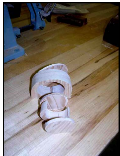
Drawers for the above box are cut by making a "U" cut as in the second piece from the front. Cut the back off, then cut out the drawer piece, cut off the front and back, cut the "U", put it all together again.
