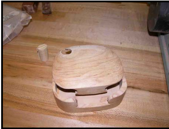
No, I am not going to try to document this one, but suffice it to say that the little peg locks the box, and it SLIDES open instead of lifting off. Sort of a Puzzle box!
