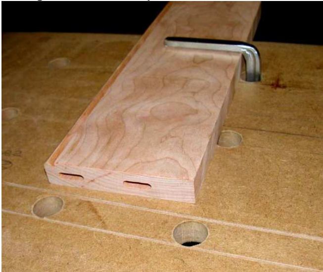
Slots cut in this end, the piece is reversed, face up, with proper orientation for cutting
