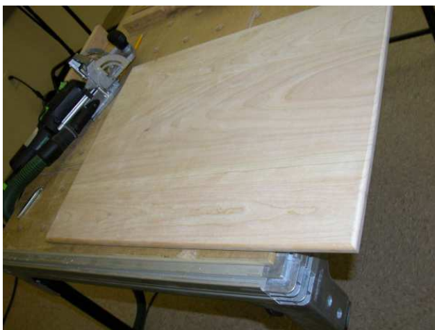
Angle of this shot is a little weird, but the table top was made from portable tools except for the surface planing.
