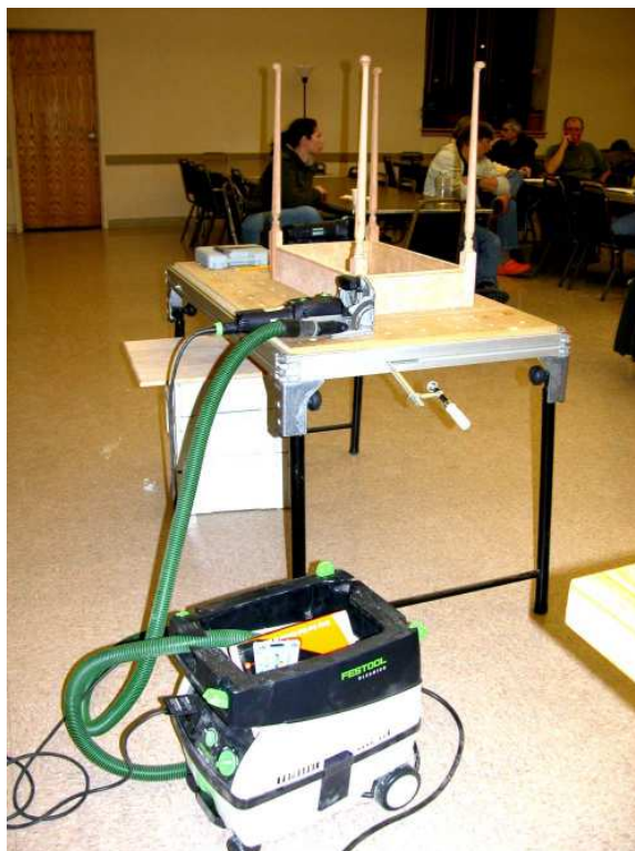
The setup – Festool Domino hooked up to a Festool vacuum. Work held onto Festool work table with Festool clamps. The extension cords I do not know.
