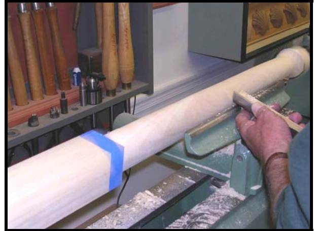
Turning the main leg shaft. Note the use of blue tape at the end of the pommel.
