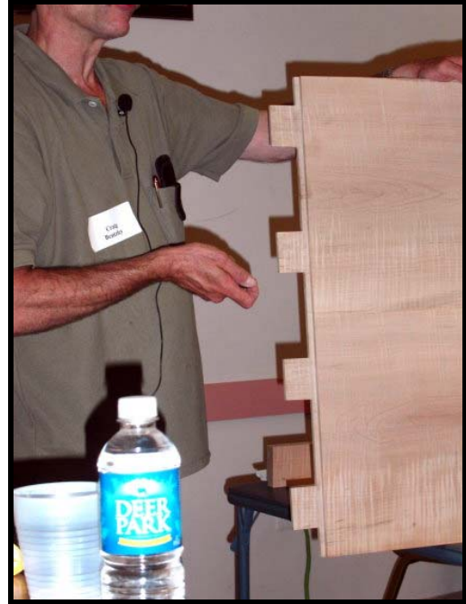
An even better look at the tongues on the breadboard end of the table.
