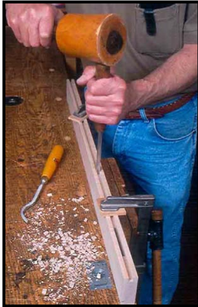
Hand cutting the mortises in the breadboard end.
