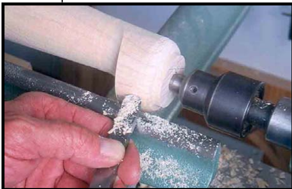
Finishing the foot and foot pad.
