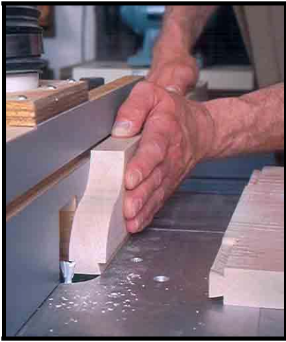
Routing the dovetailed sides of the cleats on the router table.
