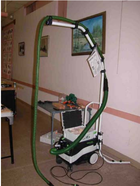
A new addition to the Festool system (well I never saw it) is the arm that lifts a long dust collection hose overhead and out of your way, Nice feature and hooks right up to the Star Wars style vacuum.
