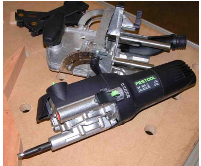
The Domino taken down, showing the cutter on the lower right and the fence, much like a Biscuit joiner fence, in the top of the photo. This comes apart very easily for cutter changes and adjustments.
