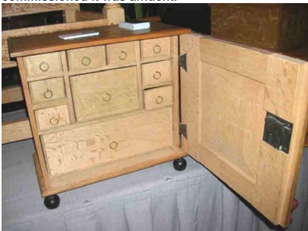
The inside of the cabinet shows (if you look REAL hard) that the way to find the middle of the drawers was to scribe two diagonals on the fronts. But – they never bothered to remove the scribe lines, and these were left in place.
