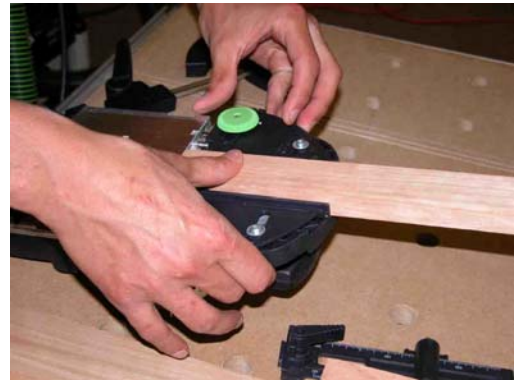
This accessory is included with the slightly higher priced kit. It allows you to put the dominos in narrow pieces.
