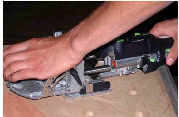
Looks like a biscuit joiner. Not hardly. Here, the motor is being re-fit to the front end of the tool.
