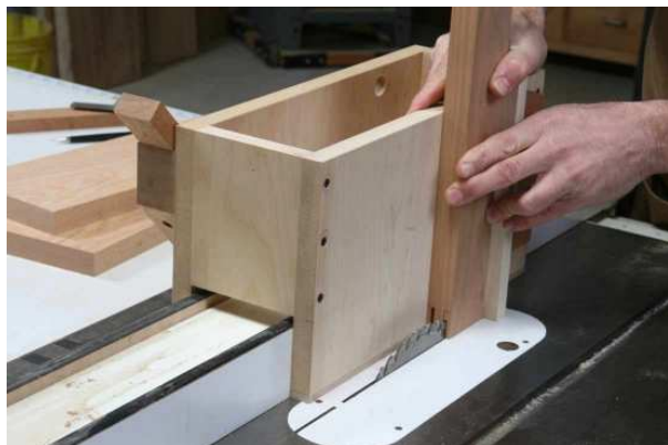
Tenoning jig in action. Rides a square fence.
