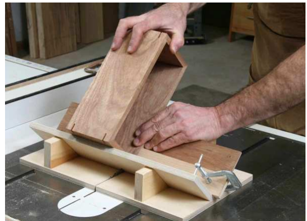
The jig in use. Note the spacer clamped in place for consistency.
