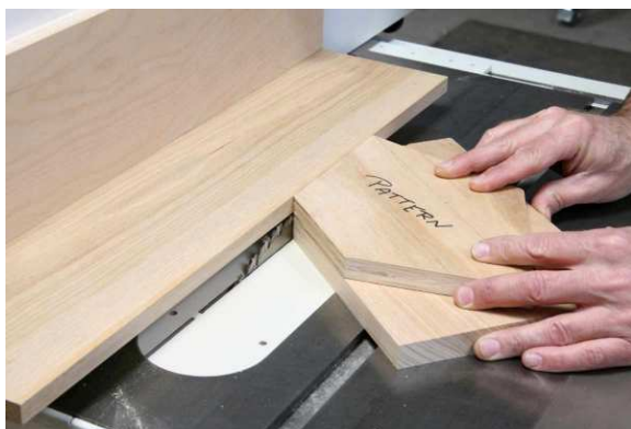
Pattern on top, work on bottom. Double face tape works well here. Pattern follows edge of jig.
