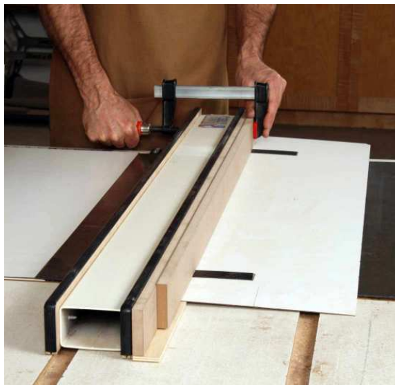
The setup for the thin stock cutting fence. You can see that the laminate runs under the hold down fence and above the leg of the "L" shaped fence.
