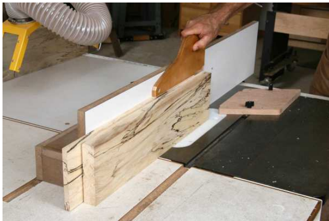
This tall fence does the trick for resawing operations.
