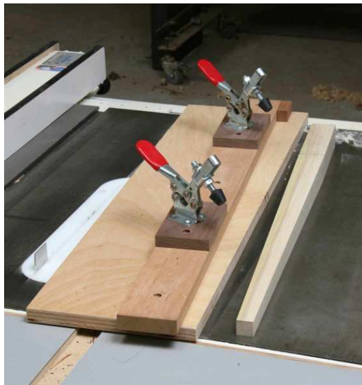
Tapering jig. Bottom is a piece of plywood. Toggles mounted high on blocks that are affixed to a pivoting jig with a stop block on the end.
