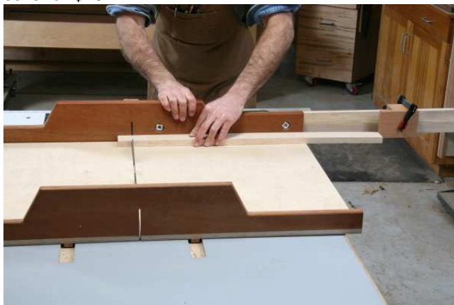
IN use with the extension arm and stop block.
