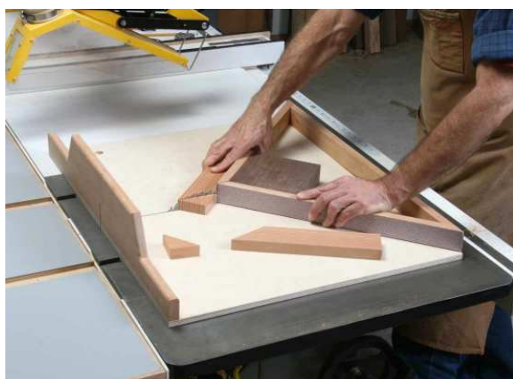
This miter jig, made properly, greatly enhances your ability to painlessly make accurate frames and miters.
