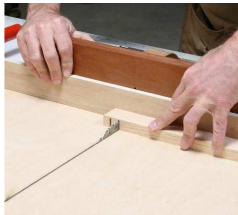
Set blade depth, put wood against brad. Make a cut. Slip wood over brad into first cut, Make a cut. Again. Again.
