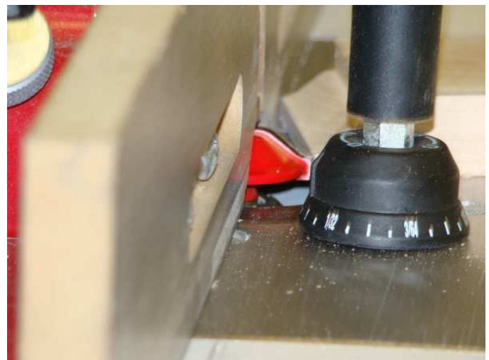
Here the end piece is turned over and the top edge of the bit, where the radius starts, is aligned with the edge of the work. The really neat micro adjust knob makes it easy on this mini table Jason used a couple of times at our guild.
