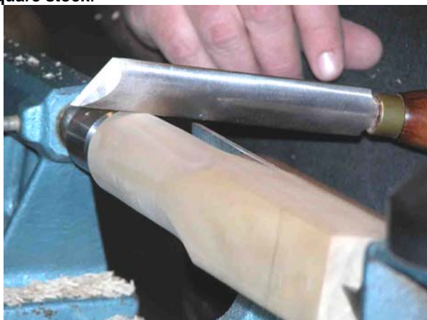
Several items to note – the skew has an oval shape rather than a flat shape. Second, the tip is beveled, not square. See the text as to why a skew of this shape was chosen for use. Lastly, this lathe is actually running and bill is holding the skew on the round piece – if it bounces, there is more work to do.
