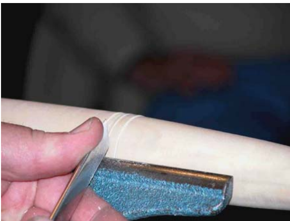
Making the center leg detail with the tip of the skew.
