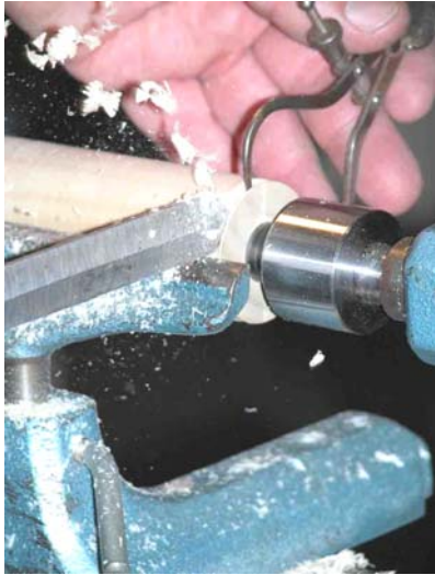
Use of the caliper in getting the foot end diameter. Remember to leave material for sanding,
