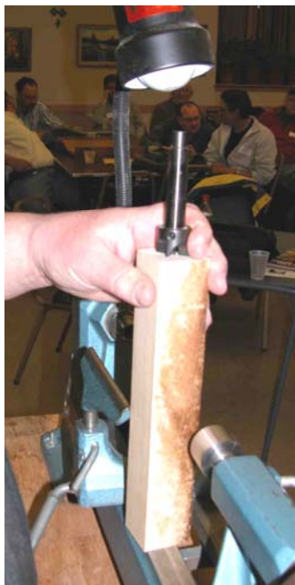
Bill cautioned that you do NOT drive the head end into the wood while resting on the lathe ways or bed – they can crack.
