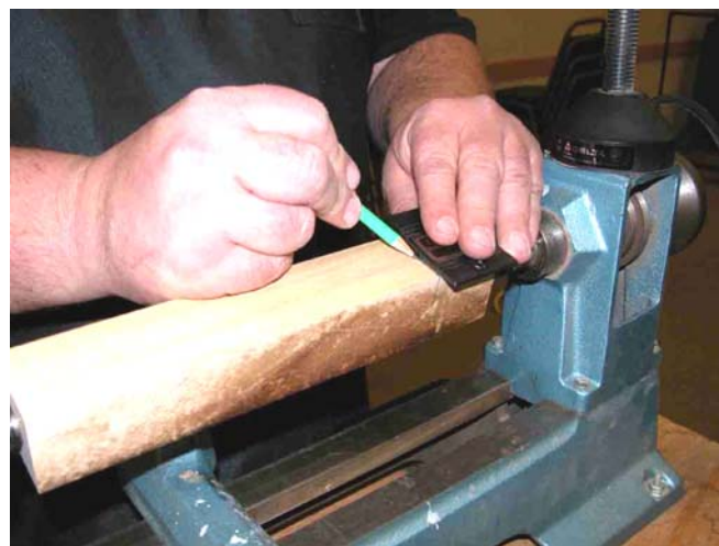
A right angle square Bill uses to mark the pommel end.
