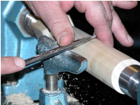
Dampening harmonic oscillation ala Grumbine.
