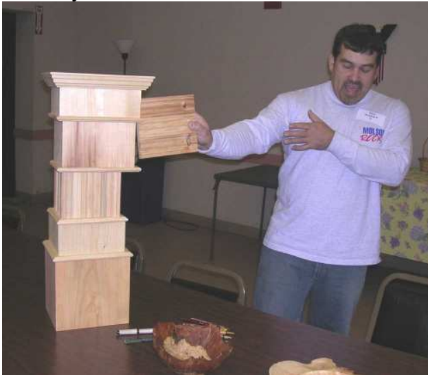
Russ got a commission to build a replica of an 8' high mantle. The pieces go together vertically like the stack he has, and the cross piece he is holding. Close up you can see how much detail is in it.
