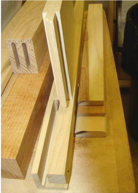
Here are some examples of how this can be used to cut mortises for table aprons and the like.
