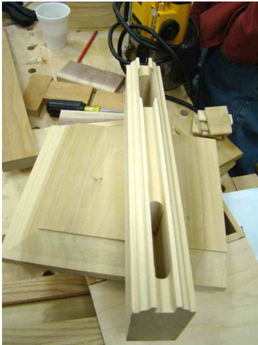
An example of a few things here – first, the versatility of the sizes you can work with using this setup and then how you would use it to strengthen cope and stick joinery. For this you use a tenon the size of a small brick. Actually, 3/4" thick by 5 3/8" long.
