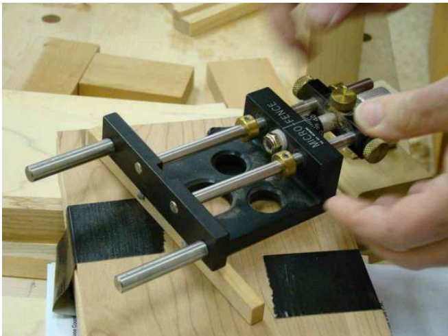
This is the Microfence with the guide strip attached as you can see. Note the many fine adjustments and the stop collars in the center.
