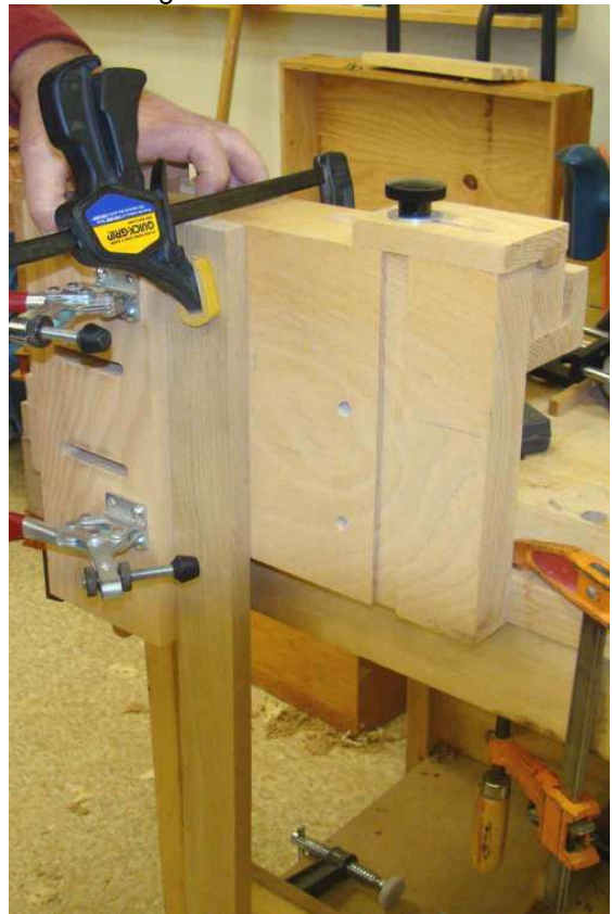
The stoc k in place for an end cut. The Quick grip temporarily holds it while setup is done initially.
