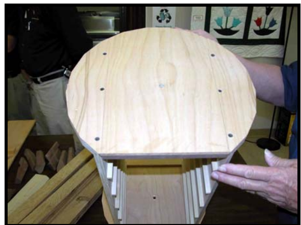
This photo shows the segmented top of the chest. Ken designed a jig (next photo) to make consistent cuts once the layout is penciled onto the work.
