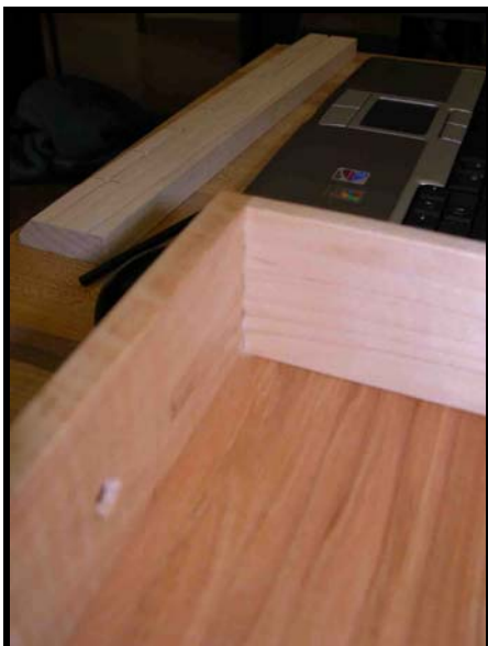
But inside, you cannot see any indication of the finger joint construction.
