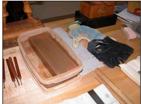
A water stone, some micro gouges on the left, and protective gloves to the right.
