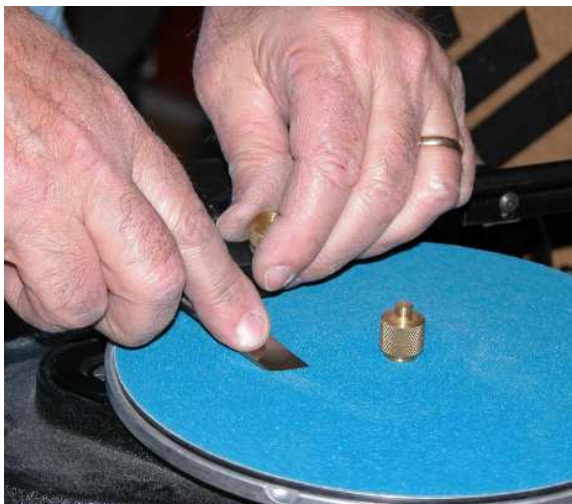
Bill at work on the Veritas. As explained, 2 disks are included of differing thickness. Moving from the 4 mm disk to the 3 mm disk for finishing gives you the microbevel. Abrasives of differing grits can be used on either side.
