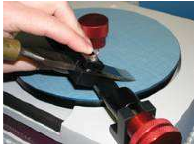
In use with the optional guide bar/ Many accessories are available, and the machining of this is totally top notch. There is also a wet system for it with a rubber collar to hold water.
