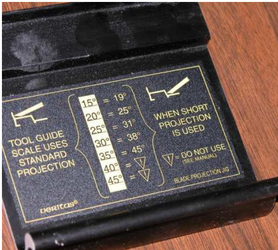
This jig attaches to the guide bar on the Veritas and shows setups for desired bevels.
