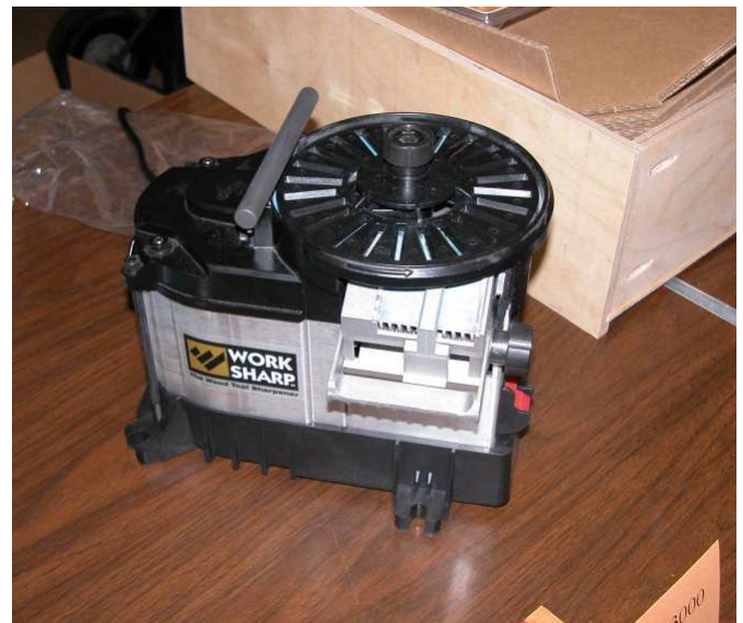
This is what the unit looks like. In this photo, the perforated platen is attached and you can see through it if you want to see the sharpening.
