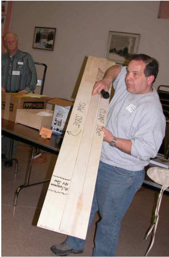
Gerry demonstrates his circular saw cutting jig.
