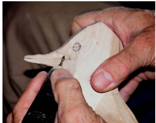
This part was pretty interesting – he used the fine grinder to cut the line where the top of the beak meets the face.
