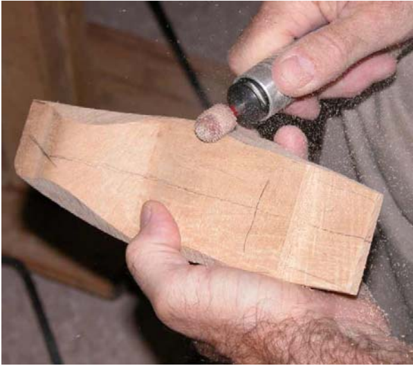
Rounding out the blank with the heavy grinder. This one removes stock very fast. Note – unlike knife carving, you will make a lot of very fine sawdust with this method and should use both dust collection and breathing masks.
