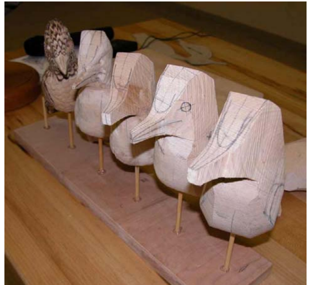
This photo shows the series of steps that a blank takes (right to left) until it becomes a bird.
