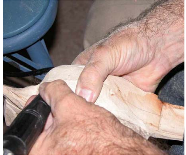
The fine detail grinder is used to outline the feathers on the breast. A scalloped design, that must be done randomly for realism.
