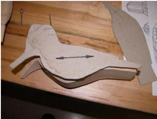
The side is traced onto the blank and that profile is cut on a band saw. Not that on this piece there is a reference arrow showing the direction that the wood grain should go in.
