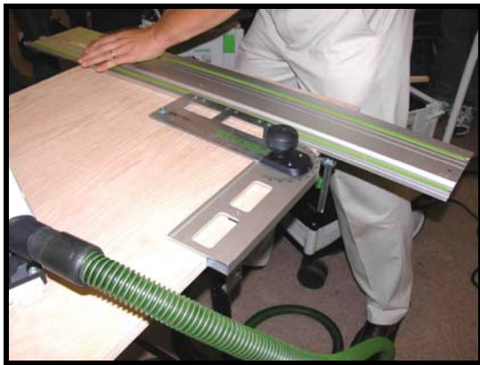
Another style of miter gauge that can be used without the work table.
