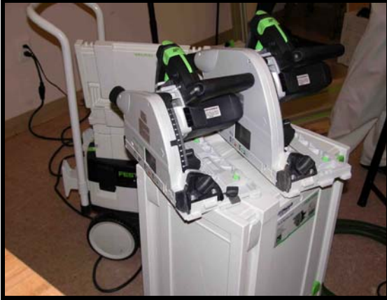
Dust collector in the rear with Systainer on top, and a large sized Systainer in front with circular saws on top.
