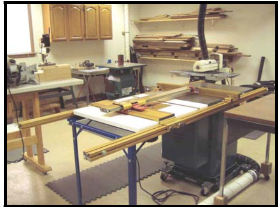
Terry loves his Inkra fence and extension table mounted router. Terry advised it takes a long time to set up but is worth it. Table saw is a 3 hp, 10" model. Router Terry uses in the side table is a 3 1/2 HP Porter Cable.
