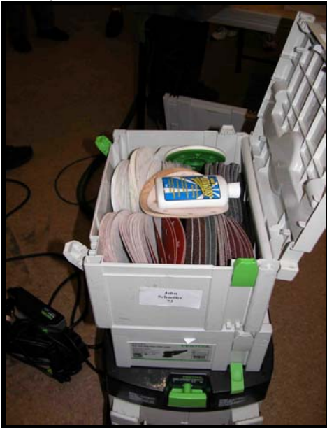
At the sanding demo, a Systainer sits atop of the dust collection unit and hold sanding accessories.
