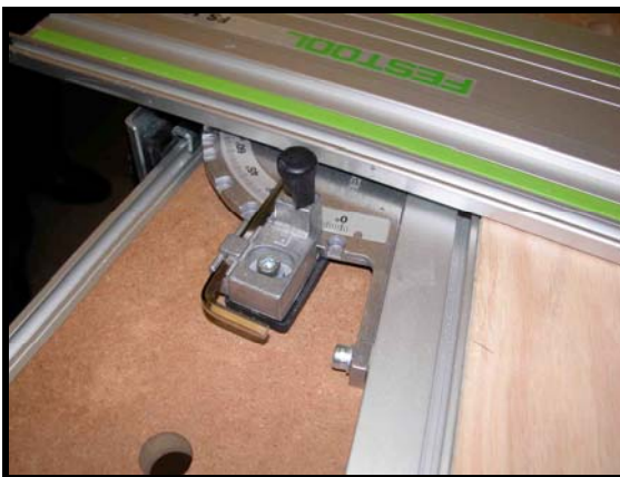
A shot of the miter gauge that comes with the table, the elevated guide rail stock can slip underneath. Saw rides on guide rail, almost simulating either a radial arm saw or a compound miter saw in function.
