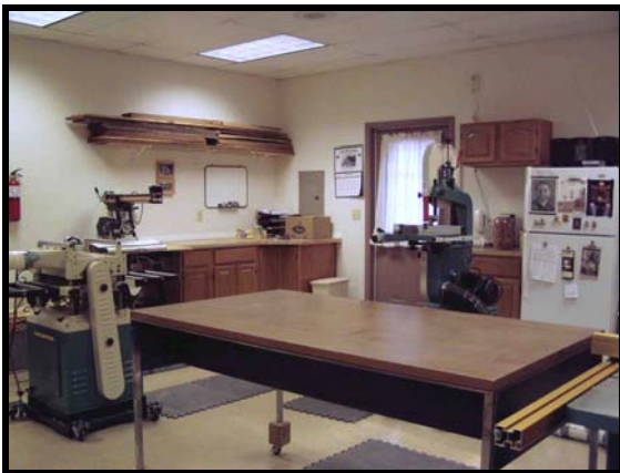
Looking to the other side, refrigerator provides refreshments and has radio on top. Radial Arm saw on left, 14" band saw next to fridge. All items are on wheels, as Terry uses this shop as a party room when needed. Rolls everything out the double doors! Fire Extinguisher is mounted near the fridge, There are 4 ceiling mounted speakers, handy when parties are in swing. Phones are hooked up to flashers so Terry can tell if they ring while he is using noisy equipment.
