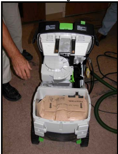
The Dust Extraction unit – guts view. Disposable bag.
