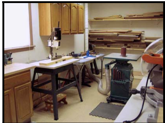
Drum sander, mortise machine and, on right, chop saw station. Nice spacing between tools everywhere in this shop. No clutter = safety. Terry did a scaled mock up of the shop, with scaled pieces of paper for shop tools, arranged everything on the template before breaking ground. He allowed for expansion in his plan. No extension cords are needed as he installed loads of 20 amp outlets, and the building is on a 100 amp service.
