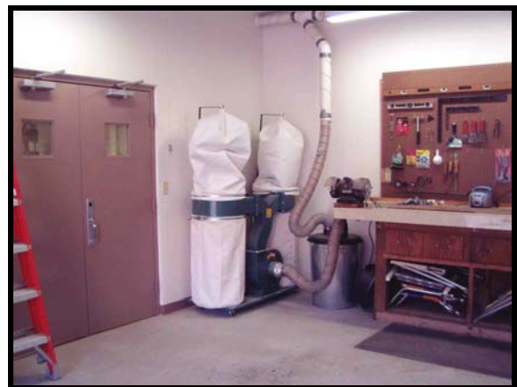
Terry's 3 hp dust collector is outside of his shop. Keeps noise down in the shop. Easier to empty outside. Double metal fireproof doors salvaged from a construction site.
