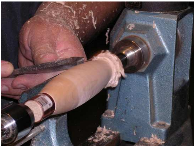
The ferrule on the work, Bill turns (HA!, get it?) his attention to the butt end of the tool.
