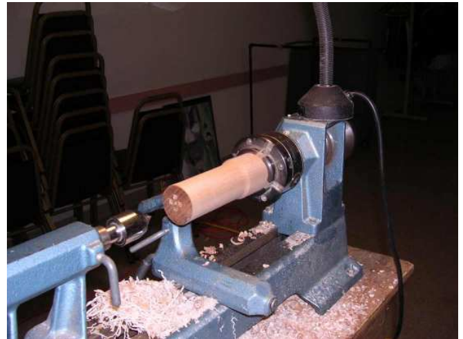
As I think they used to say on Hollywood Squares, "the square gets a circle!" The square blank is round and Bill checks for roundness by turning on the lathe and laying a tool over the top of the work. If it judders, the work is not round. This photo happens to be from the second handle Bill turned.
