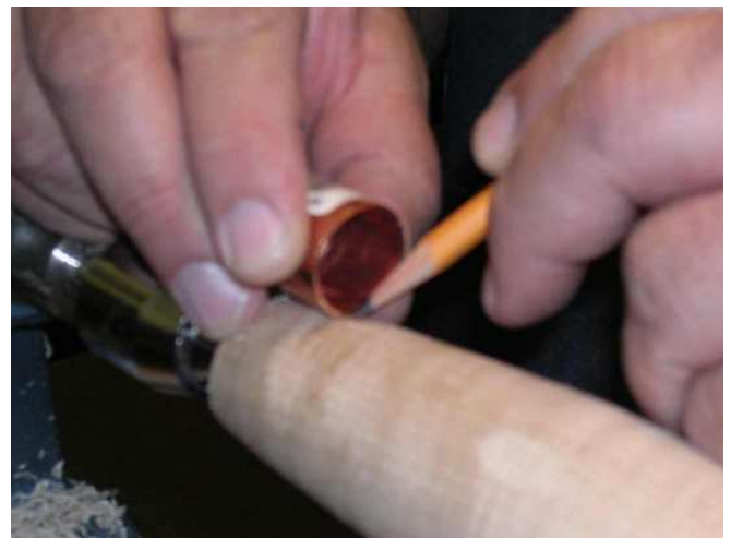
Bill was careful to mark the work with the length of the ferrule before doing this. Bill uses a caliper to measure the diameter, but cautions to turn OFF the lathe and not attempt to measure while it is running. Embarrassing to have a caliper sticking out of your forehead in the Emergency room.
