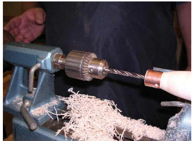
Here Bill has removed one of the centers on the lathe and replaced it with a drill chuck that slips into the lathe. He has installed a bit of proper size, gently moves the drill bit point to the center of the handle, turns on the lathe, and cranks the center with the chuck mounted into the handle to the proper depth.
