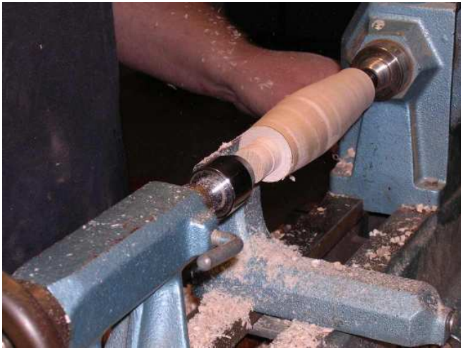
The work is now to the point where Bill used a parting tool to get the shoulder close to ferrule diameter.
